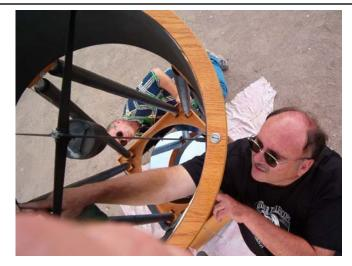
**Joe and Ron collimate** Joe Hillberg and Ron Hoekwater adjust the primary mirror to complete the collimation of the Starsplitter.
