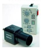
purchase price. Connecting the camera to the telescope is very easy. A 1.25" C adapter screws into the front end of the camera. The Stellacam II has no lens and operates at prime focus. Once the C adapter is attached the camera simply slides into the telescope's 1.25" opening. A composite video cable attaches the back of the camera to the back of the monitor via BNC and RCA connectors.
