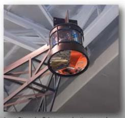
Large Binocular Telescope adaptive secondary incorporating 672 voice coil actuators
